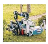
algorithms that enable the robot to compare overgrown bushes with ideal final shapes as it trims. Using a different cutting tool, Trimbot can prune roses by pinpointing the exact part of each plant's stem that should be snipped.
