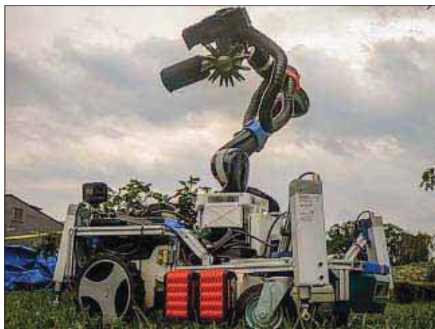
The Trimbot is armed with a toolkit of blades and a flexible arm and makes short work of gardening chores
