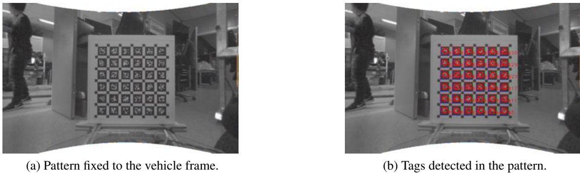
Figure 5: Estimation of camera to vehicle transformation.
