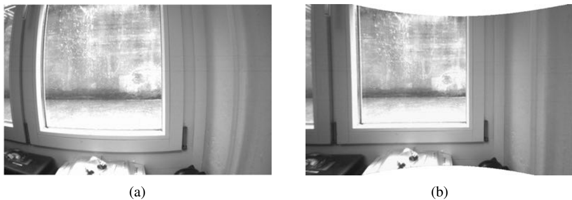
Figure 3: (a) Raw image of a single camera from the pentagon setup. The distortion effects of the lens are visible as the window frame is curved. (b) The corrected image with respect to the lens distortion based on the obtained intrinsic and extrinsic camera parameters.
