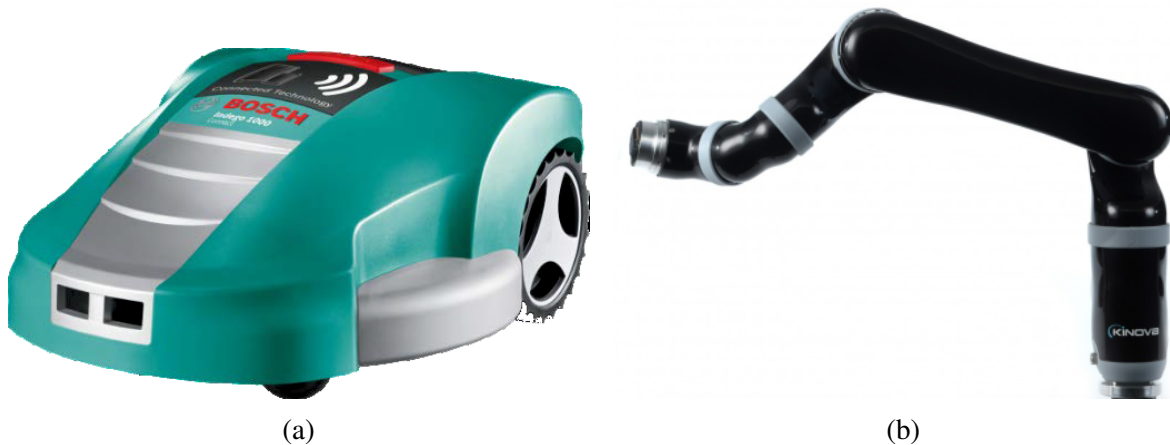
Figure 1: Basic components used for demonstrator 3 prototype. (b) Kinova Jaco 2 , (a) Robotic Lawnmower Bosch Indego 1200.
