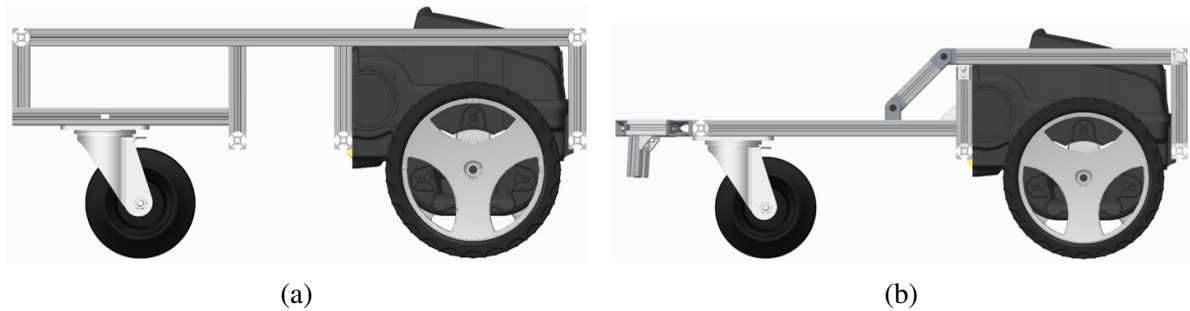
Figure 10: Side views of vehicle aluminium frame for initial and improved concept. (a) initial concept of aluminium frame (b) improved aluminium frame used for the final version of platform 3.
