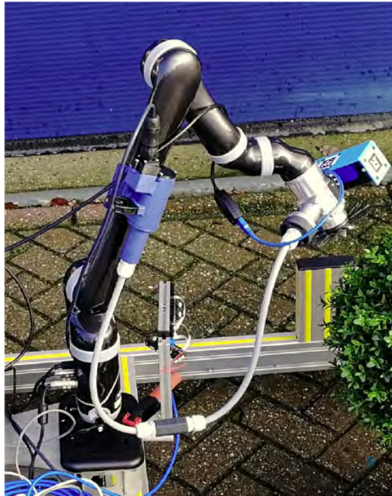
Figure 1: Realized bush trimming drive system using a flexible shaft to drive the cutter tool
