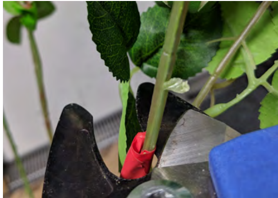
Figure 18: Result of the visual servoing where the end-effector reached the target with the tool in the centre of the target.
