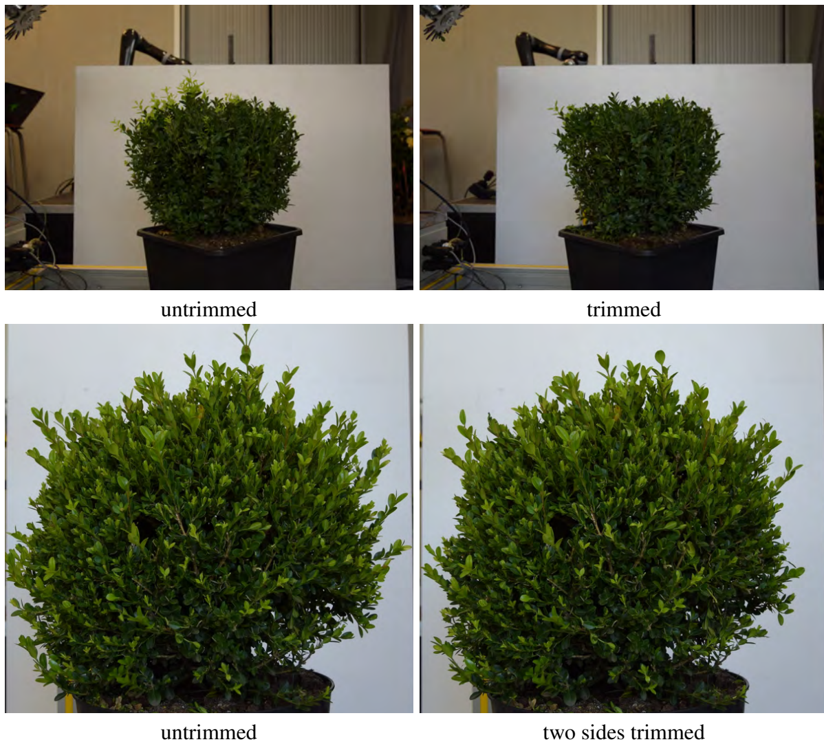
Figure 10: Top: Trimming evaluation of the cube bush with outgrowth. Bottom: Trimming evaluation of a spherical bush with significant outgrowth. After one trimming step, the bush was rotated by 90^\circ and re-scanned. A new trimming trajectory was planned and executed, after which the bush was scanned once more. The top images show that outgrowth was removed on the left and right sides, but not all branches were caught by the trimmer.
