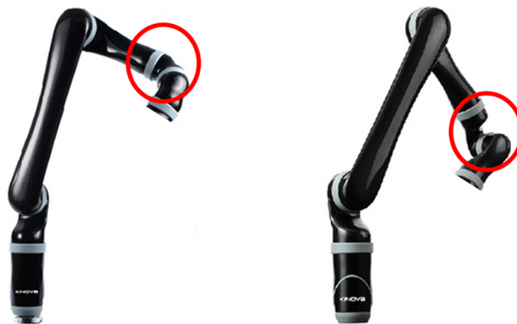
Figure 1: Kinova Jaco 2 configurations with curved wrist (left) and spherical wrist (right).
