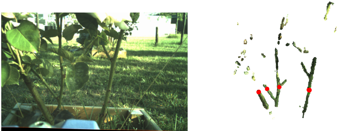
Figure 11: Rose clipping site detection. One image from the bush scan set (left) and corresponding detected clipping sites (red) on the segmented pointcloud of the bush (right).
