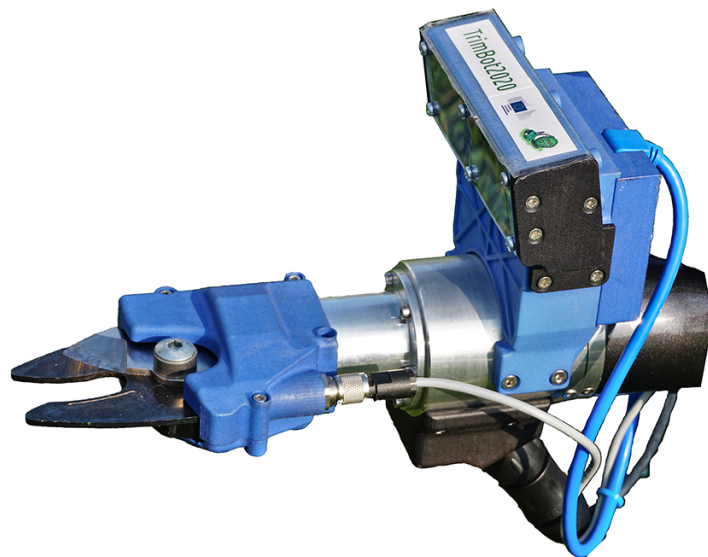
Figure 10: Photo of the final version of the rose clipping end-effector.
