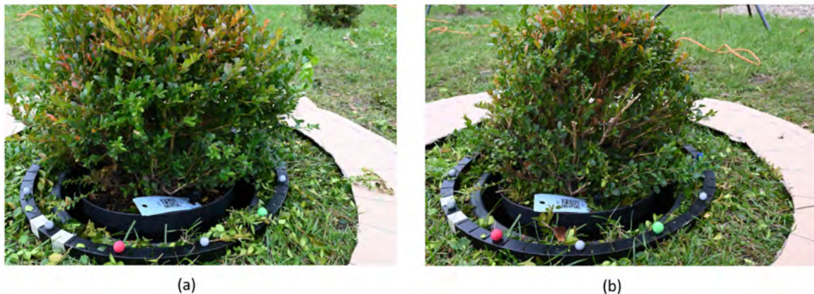
Figure 11: Showing a sphere before (a) and after trimming (b). At some poses the robot trimmed too deeply. This can be observed in figure b since here the inner branches are visible.
