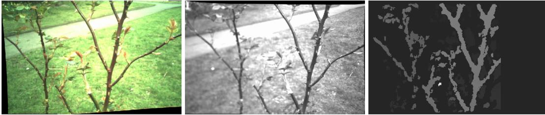
Figure 2: Left, right and disparity map obtained by the stereo camera.
