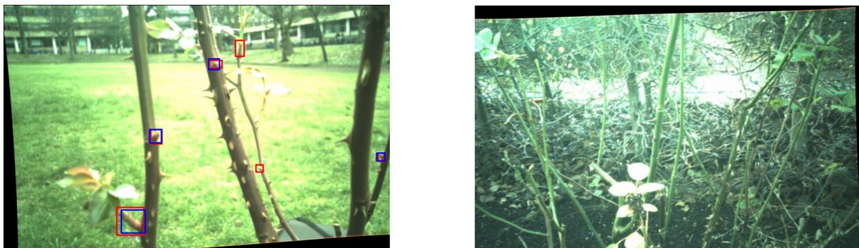
Figure 8: *Left*: bud detector inference results (blue) on dataset compared with the ground truth (red) on a rectified image from the arm camera. *Right*: No buds detected because the camera is too far.
