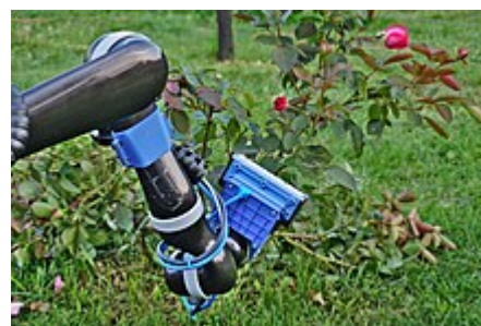
Rose cutter of the TrimBot2020 robot in action
