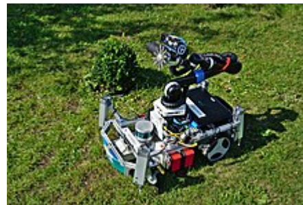
TrimBot2020 robot equipped with the custom bush trimmer end-effector.
