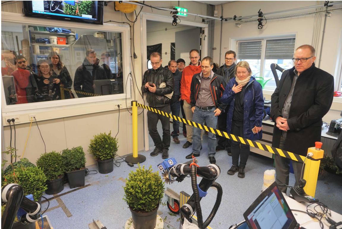
Figure 1: The TrimBot2020 bush trimming prototype (Arm and tools V2) approaching a spherical bush during the live demonstration.
