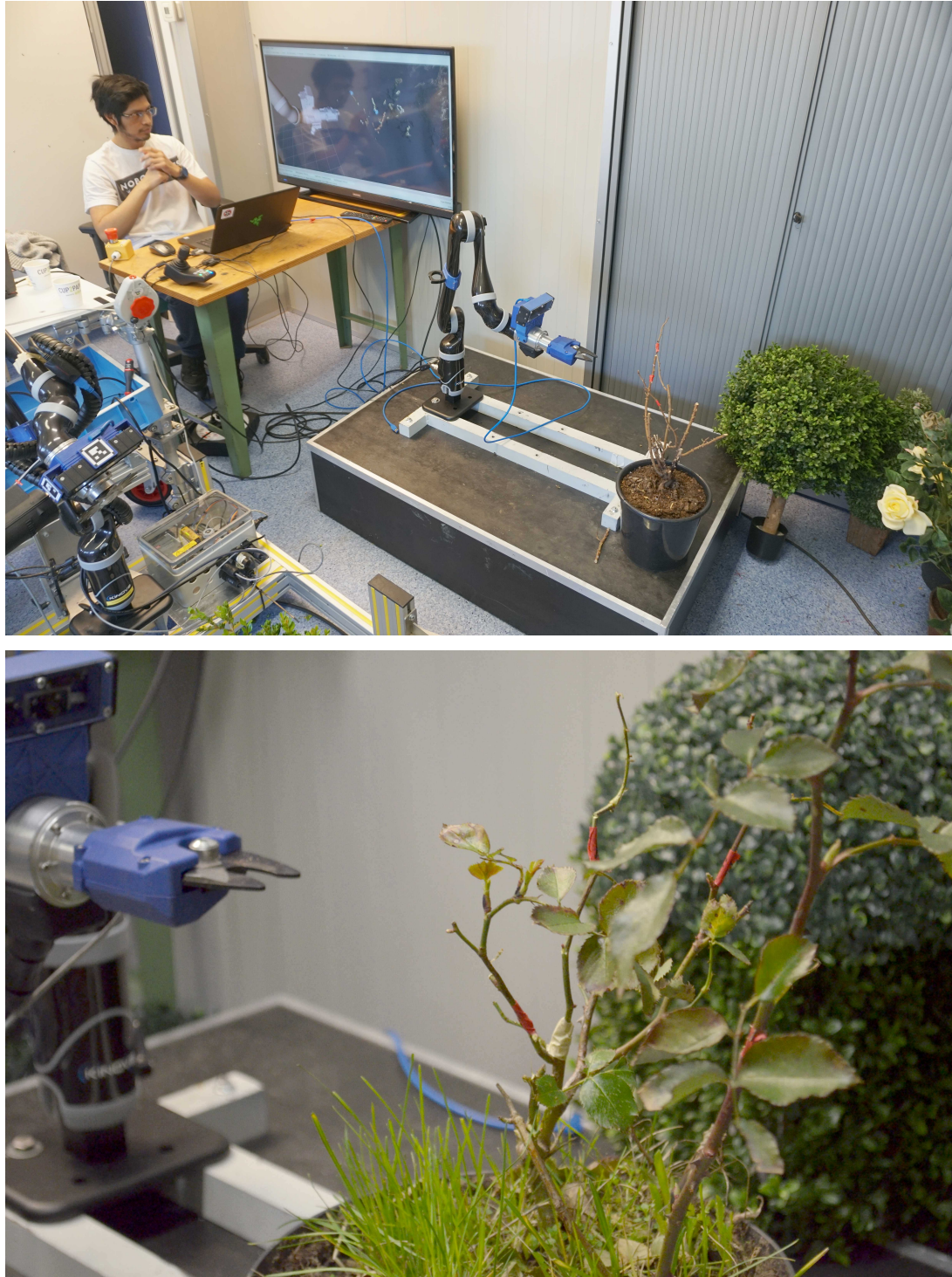
Figure 3: Demonstrator 2 setup for rose bush pruning (top) and detail of clipper approaching the bush (bottom).
