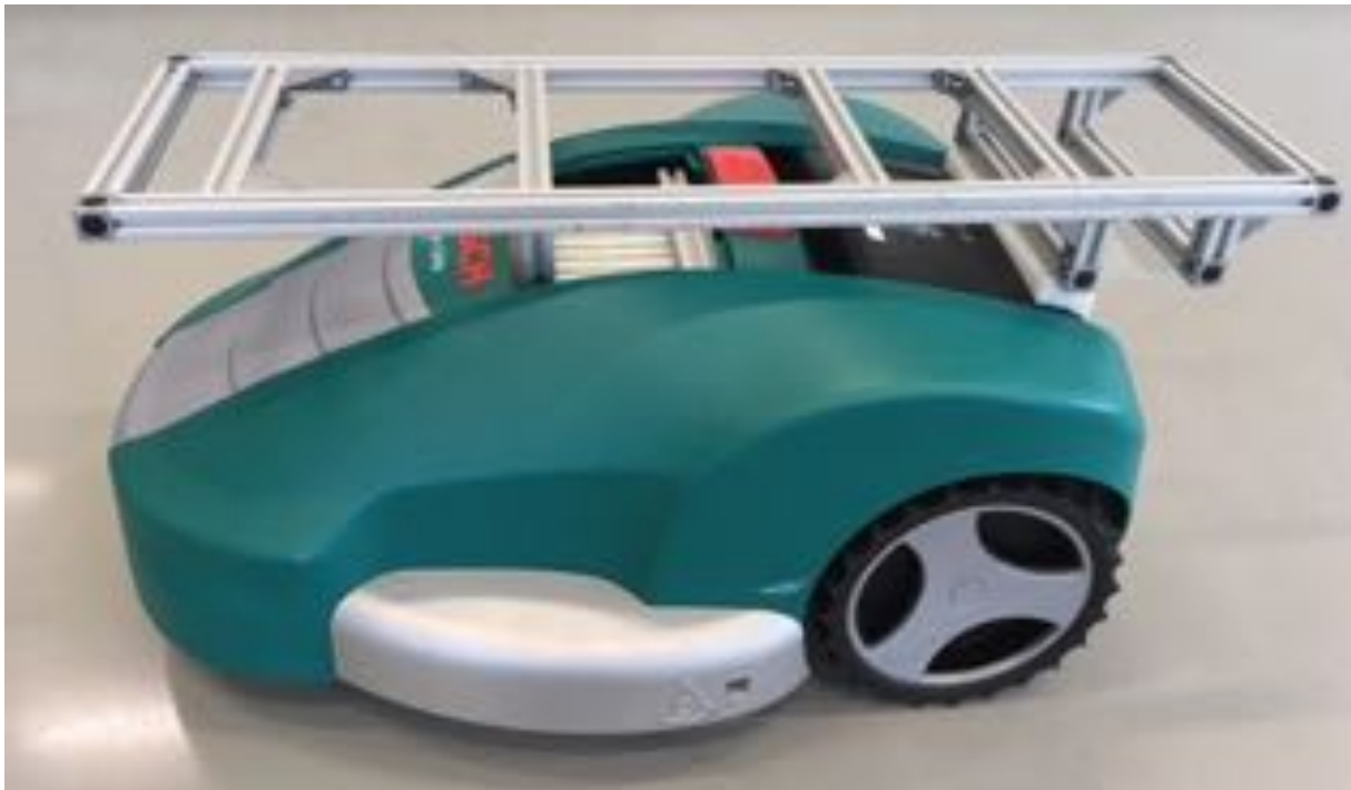
Figure 1: Aluminium frame for vehicle base.
