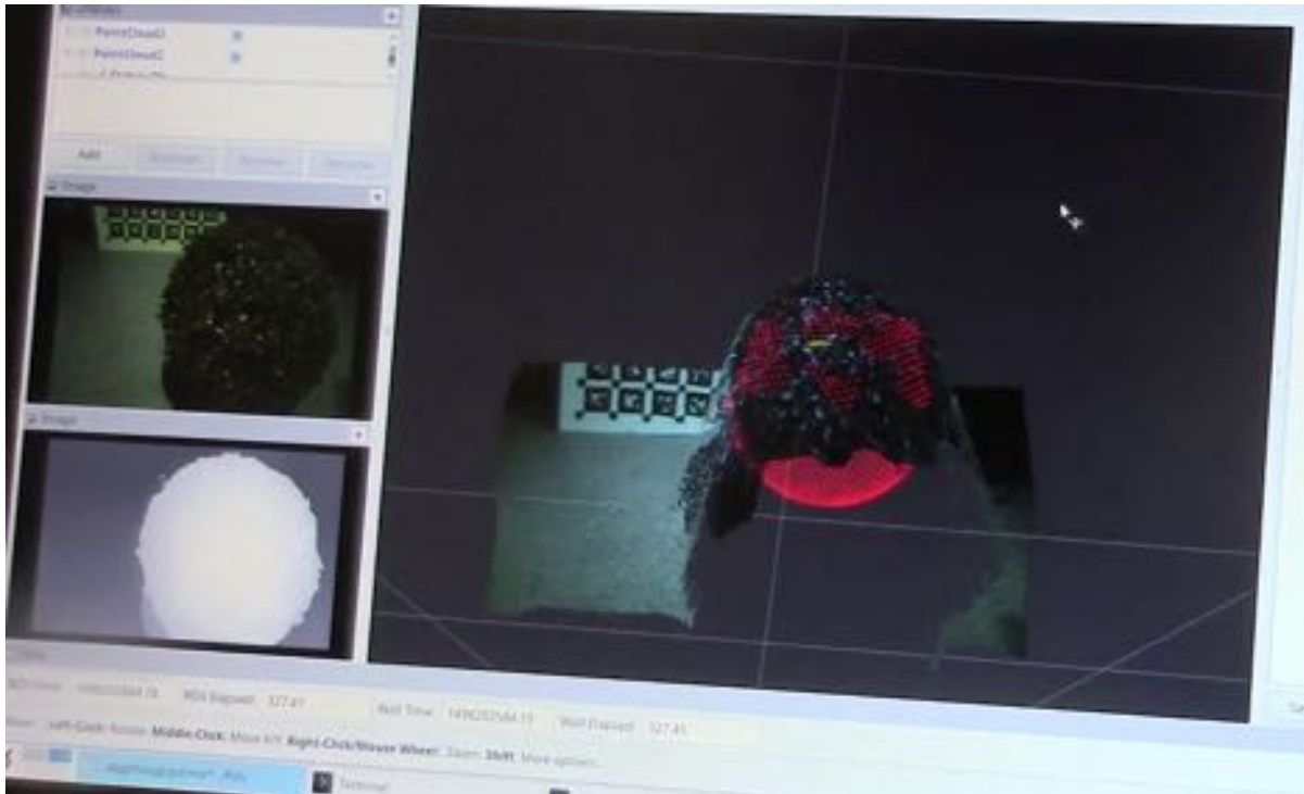
Figure 5: Vision pipeline. This screenshot of the ROS application "RViz" visualizes all the components of the current vision pipeline: On the left, the stereo camera's left image (rectified and undistorted) and the corresponding disparity map estimated by the DispNet (see Figure 4). On the right, the textured pointcloud reconstructed from the disparity map (using the known camera intrinsics) and the input image, and the least-squares fitted sphere model (shown as a red pointcloud) which tries to describe the underlying shape of the bush are visualized.
