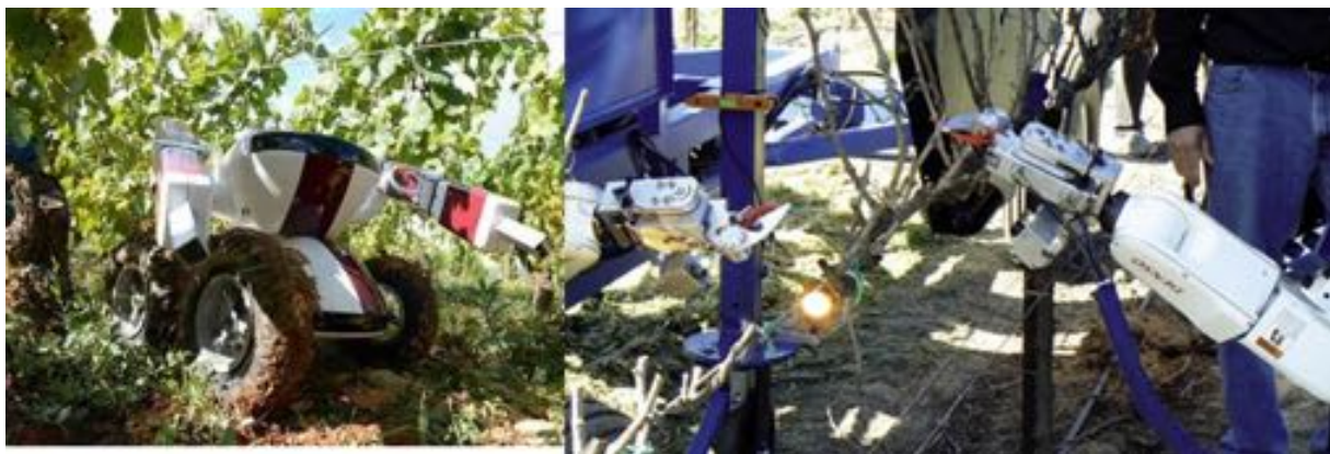
Figure 12: Wall-Ye vineyard pruning robot. Picture from: http://singularityhub.com/2012/11/26/automation-reaches-french-vineyards-with-a-vine-pruning-robot/ . Wall-Ye was developed by inventors Christophe Millot, and Guy Julien. Right, Vision Robotics Corporation vineyard pruning robot. Picture from: http://www.winesandvines.com/template.cfm?section=features&content=65505 .
