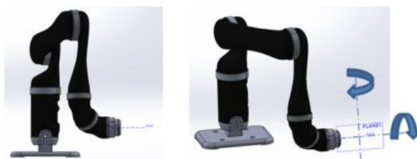
Figure 7: Left: last axis of manipulator coincides with trimming tool. Right: a planar tool would add two degrees of freedom to control
