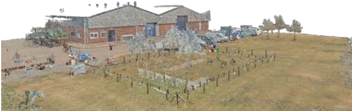
Figure 4: Detailed 3D reference point cloud with included colour data from the test garden in Wageningen. The point cloud is recorded with a Leica ScanStation P15 during the first ground truth data collection session.
