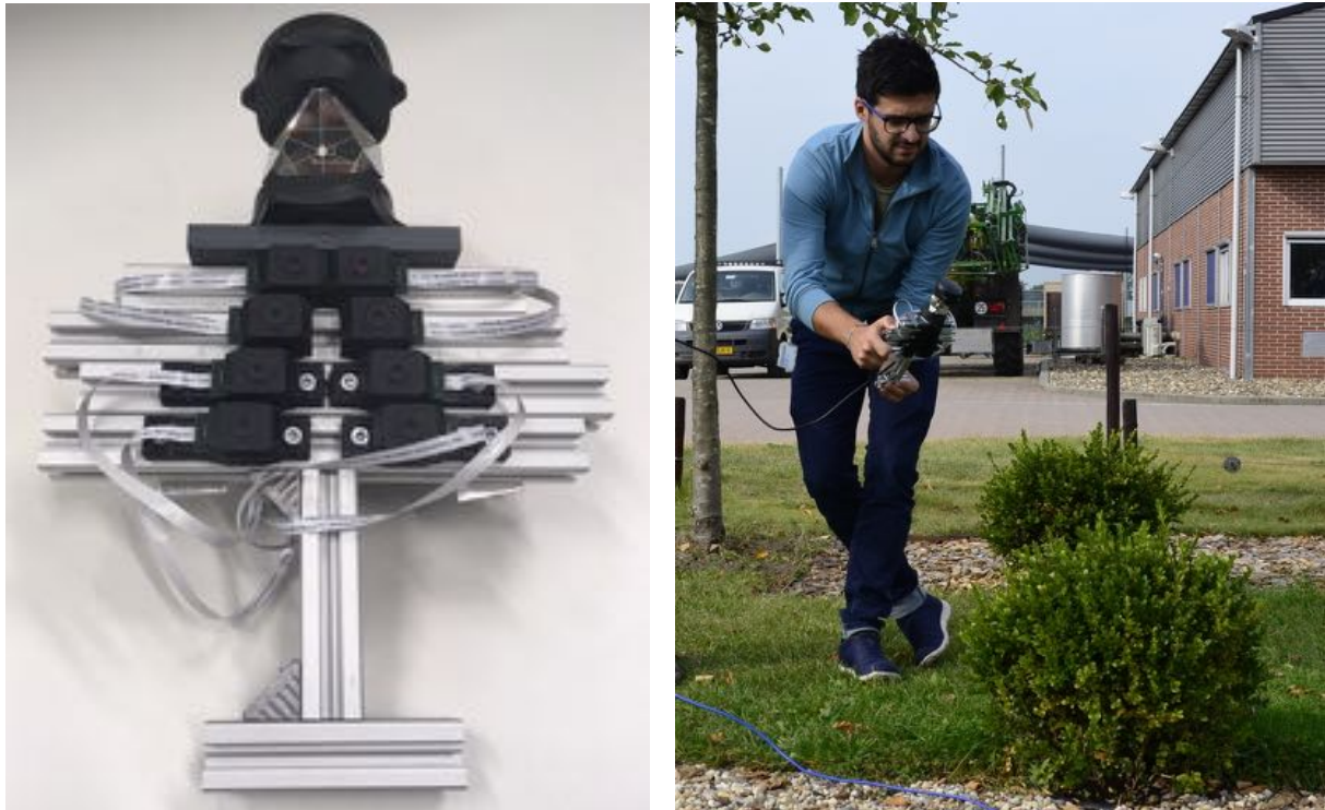
Figure 2: Handheld setup with four stereo camera pairs.
